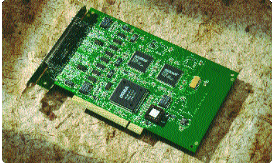
The DT340 features eight 16-bit counter/timers, 4 internal interval timers, and 32 digital I/O lines.
